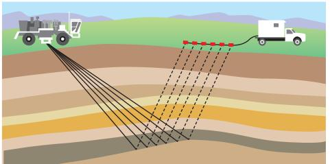
The truck on the left releases seismic waves into the ground, and the array of red sensors on the right records the waves after they have reflected off subsurface features.
