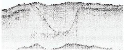
This diagram shows a profile of a buried river channel produced from remote sensing data.
