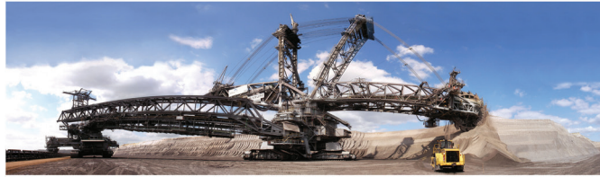
FIGURE 15.9 The Bagger 288 bucket-wheel excavator is one of the largest land vehicles of all time.
