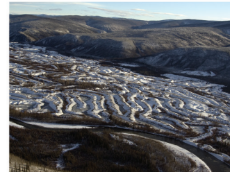
FIGURE 15.10 The sediment in this river valley in Russia has been dredged to recover platinum placer deposits.
