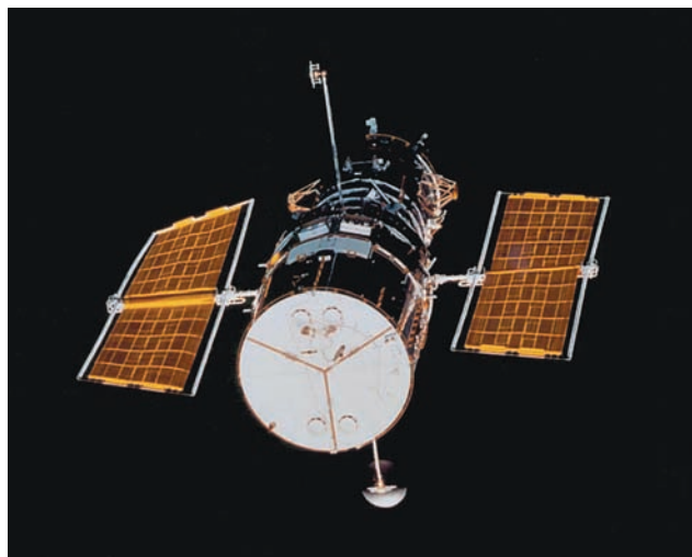
Electricity needed to operate this satellite is generated when sunlight strikes the photovoltaic cells located on its “wings.”
